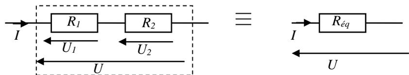
$U = U_1 + U_2 = \dots\dots\dots$       Soit:  $U = \dots\dots\dots$
