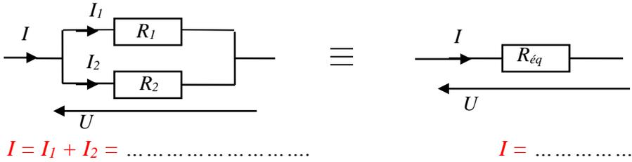
Donc:  $\frac{I}{R_{eq}} = \dots\dots\dots$                       Soit :  $R_{eq} = \dots\dots\dots$
