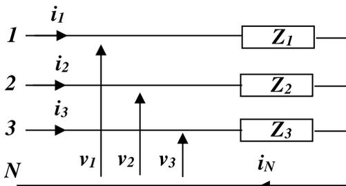
$$I_N = I_1 + I_2 + I_3 = \frac{V_1}{Z_1} + \frac{V_2}{Z_2} + \frac{V_3}{Z_3}$$
